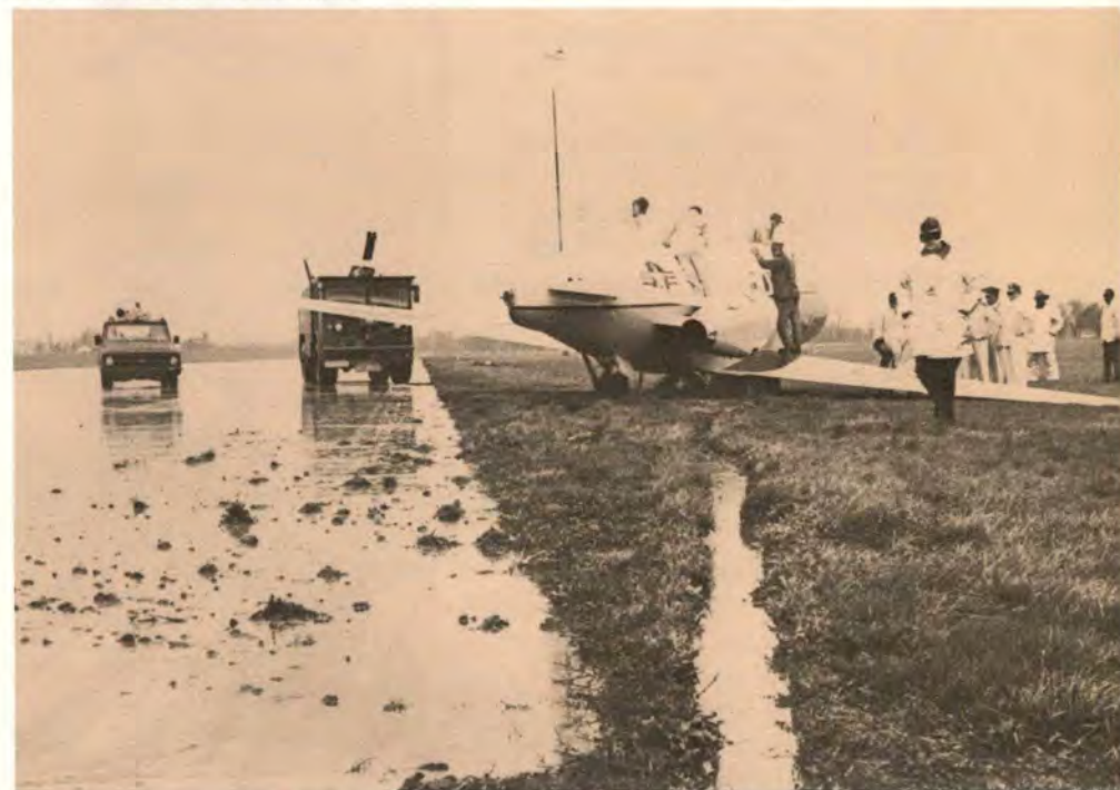
A T-39 victim of hydroplaning. A wet runway and a crosswind resulted in a skid, a blown tire, and a departure from the runway surface.
